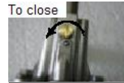
Manual Override 'ON ' Photo – 4
