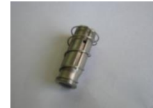
Plunger with moving seal (New Design Plunger) – Photo - 4
