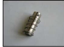
Plunger with fixed conical & cylindrical seal (Old Plunger) Photo – 3
