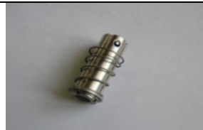
Plunger with fixed conical & cylindrical seal (Old Plunger) Photo – 6
