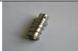
Plunger with fixed conical & cylindrical seal (Old Plunger) Photo – 2
