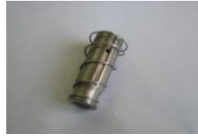
Plunger with moving seal (New Design Plunger) Photo – 3
