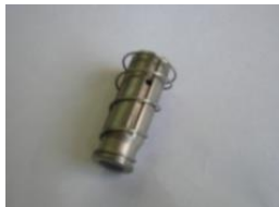
Plunger with moving seal (New Design Plunger) Photo-4
